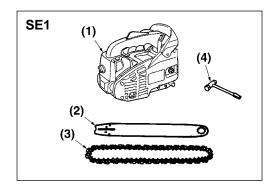
A standard saw unit package contains the items as shown below. (SE1)
